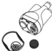
Clean the filter net (5) and filter cover (6).
