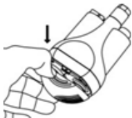
Replace the filter net (5) and filter cover (6).
