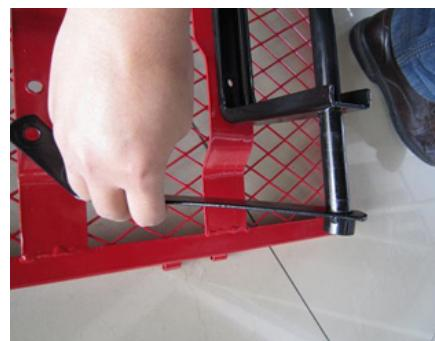
2. Align the holes on the other end of both rear axle braces (9) with the holes on the base (1). Insert M8x18 bolts (16) from under the base and through the holes. Attach an M8 washer and M8 nut (16) to the end of each bolt.
