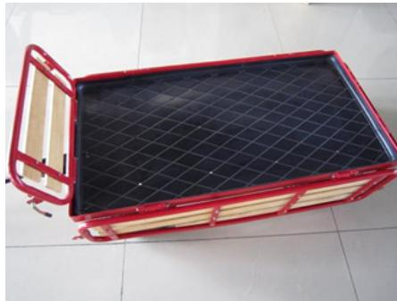
5. Pull the left side panel (2) and back panel (5) up, and turn the lock handle on the back panel (5) so that it fits snugly into the hinge at the corner of the left side panel (2).
