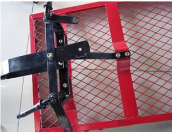
4. Place the steering brace (12) on the front axle support (10) and fork bracket (13), align the holes, and fix the parts together with three M8x18 bolts, M8 washers and M8 nuts (16).
