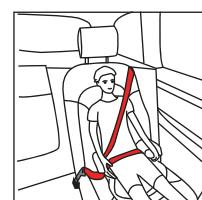
Step 3. Pull out the lap and diagonal belt and position them through belt guides with red mark. Position the lap section of the safety belt under both armrests, then insert the
